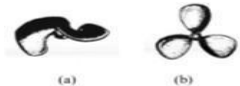
Gambar 2.16 Tipe propeller (a) propeller 2 blade , (b) propeller 3 blade
