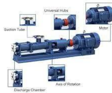
Gambar 2.29 Screw Pump
