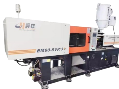
Gambar 2. 4 Mesin Injection Molding
