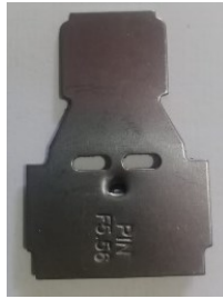
Gambar 2. 12 Proses Stempel PIN
