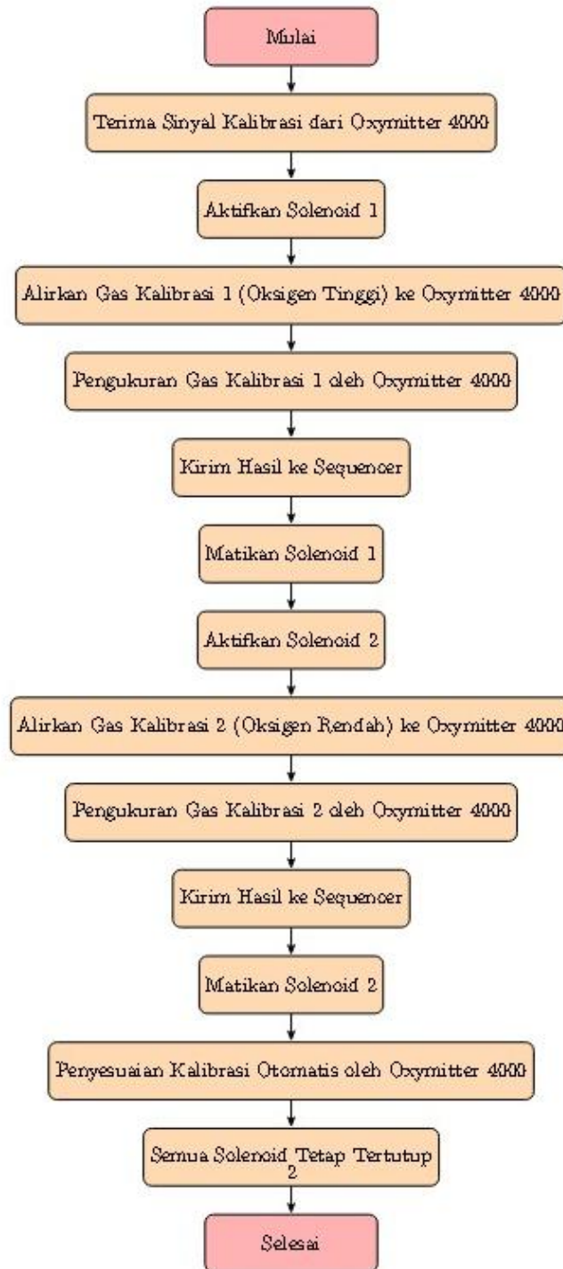
Gambar 3. 19 Flowchart Cara Kerja Autocalibration
