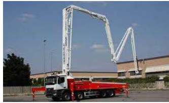
Gambar 4. 11 Concrete pump longboom
