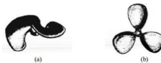
Gambar 2. 8 Tipe Propeller (a) propeller 2 blade, (b) propeller 3 blade
