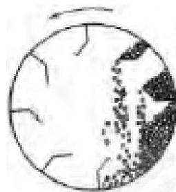
Gambar II. 34 Sudu didalam *Rotary Dryer*
