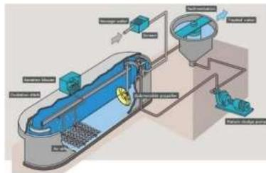
Gambar 2. 7 Sketsa Oxidation Ditch
