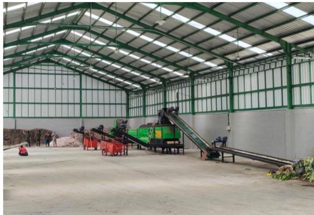
*Gambar 2. 12 Mesin Conveyor TPST*
