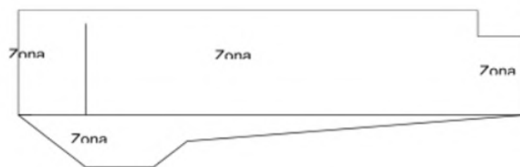
Gambar 2.6 Tampak Samping Unit Prasedimentasi
