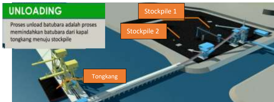
Gambar 3.1 Proses Unloading Batubara PLTU paiton unit 1-2
