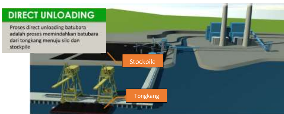
Gambar 3.3 Proses Direct Unloading Batubara PLTU Paiton 1-2
