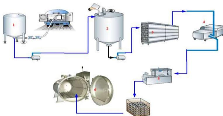
**Gambar 2. 4 Diagram Alir Proses Pengolahan Susu**
