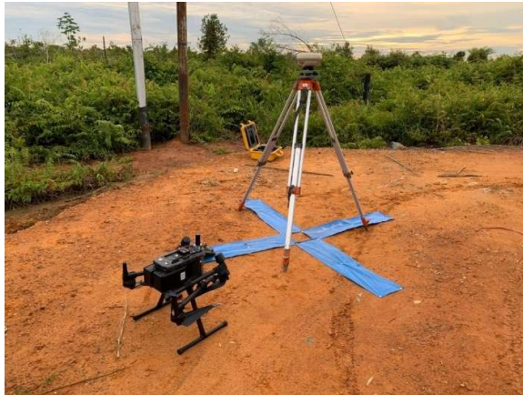
Gambar 2.8 Ground Control Point (GCP) (Sumber : TerraStore, 2021)
