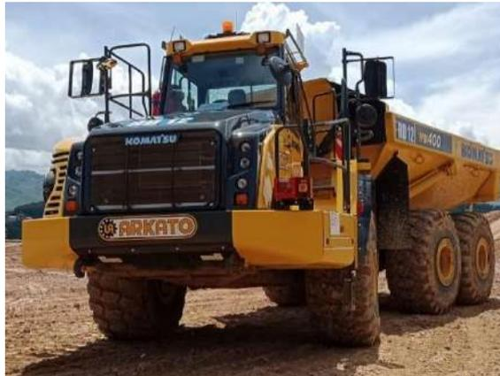
Gambar 2.7 Unit *Articulated Dump Truck*
