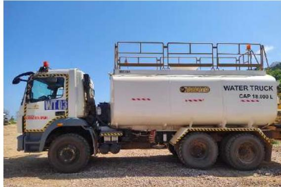
Gambar 2.4 Unit *Water Truck* Kapasitas 18K
