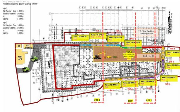
Gambar 9. 2 Denah Galian Capping Beam dan Soldier Pile
