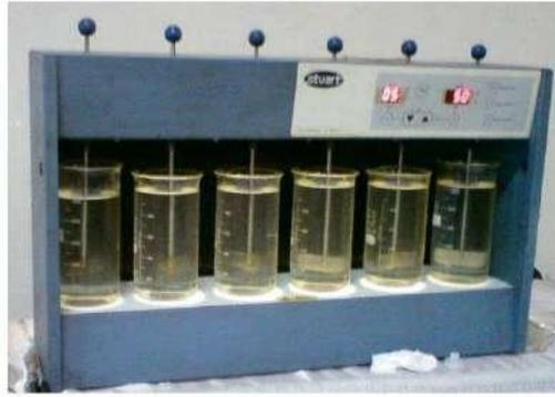
**Gambar 2.15** Peralatan Jar Test
