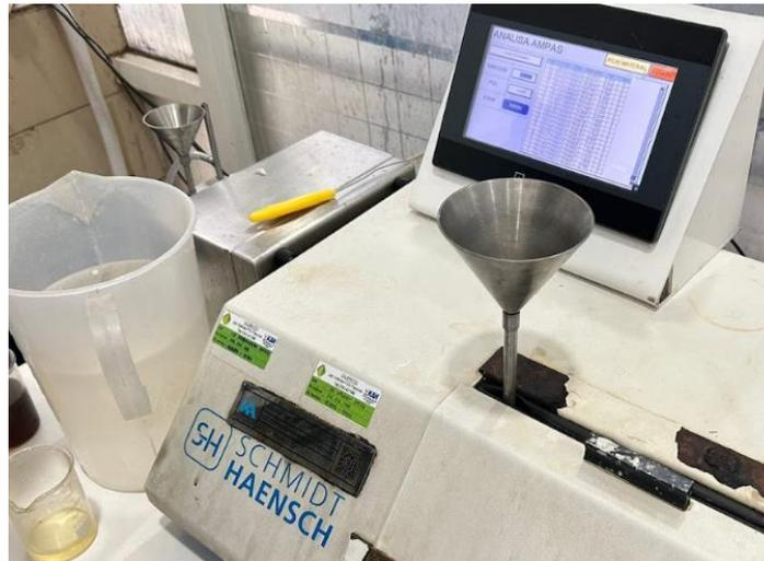
Gambar VI.1 *Refractometer*
