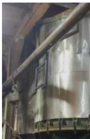
Gambar IV.12 Secondary Juice Heater
