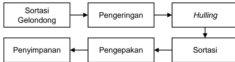
**Gambar 9.** Diagram Alir Pengolahan Kering (*dry process*)
