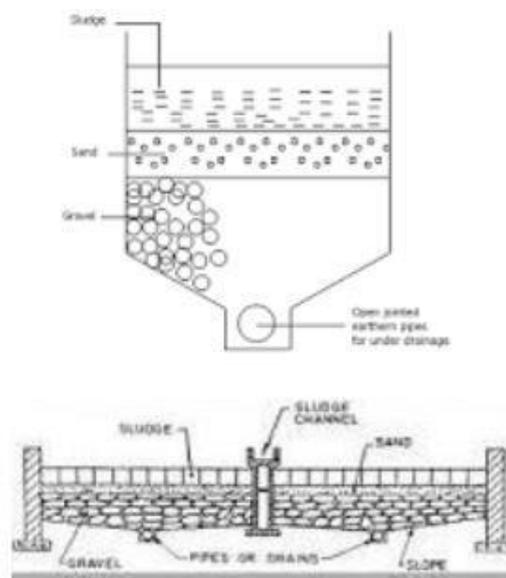
**Gambar 24. Sludge Drying Bed**
