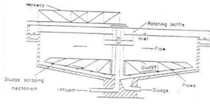
**Gambar 19.** Bak Sedimentasi Circular Peripheral Feed
