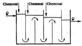
Gambar 2. 4 Baffle Basin Rapid Mixing Sumber: (Reynolds & Richards, 1996)
