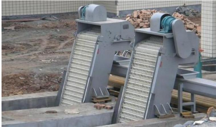
**Gambar 2. 6** Mechanical Bar Screen
