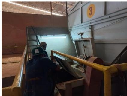
**Gambar 4.10** *Cleaning Mesin Crusher Feeder Box*
