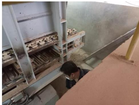
**Gambar 4.14** *Cleaning Feeder Box*
