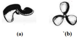
Gambar 2. 12 Tipe Propeller (a) 2 Blade (b) 3 Blade (Sumber: Qasim et al., 2000)
