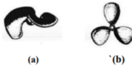
Gambar 2.9 Tipe Propeller (a) 2 blade (b) 3 blade
