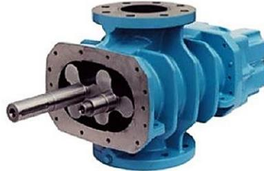
**Gambar 2.16** Blower Positive Displacement
