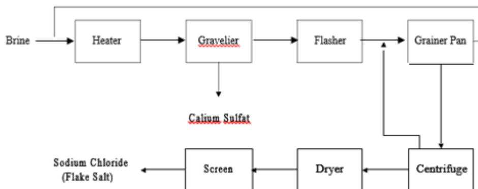
Gambar II.2 Diagram Blok Proses Grainer
