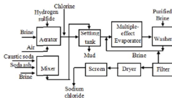
Gambar II.1 Diagram Blok Proses *Multiple Effect Evaporator*
