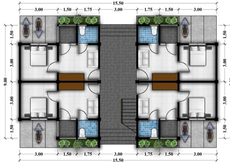
Gambar 3.8 Denah Lt. 1 type 24 generasi 3
