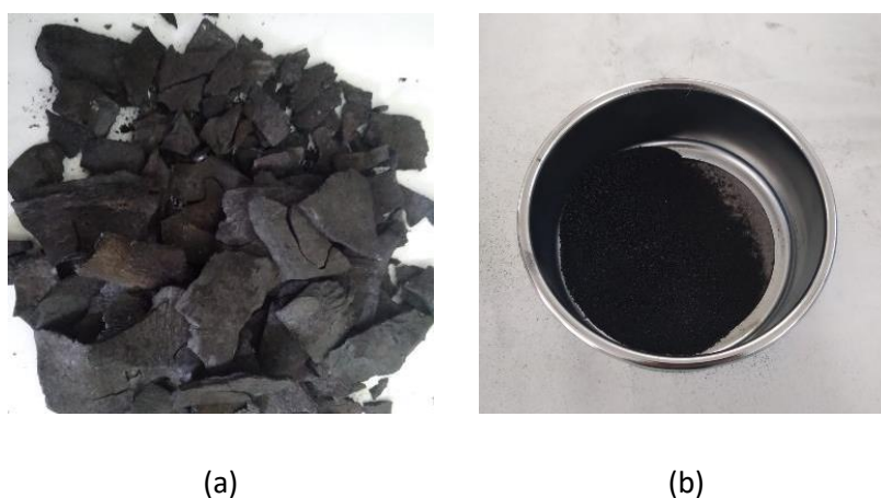
Figure 4. (a) Coconut shell carbon before crushing, Fig. 4(b) Coconut shell carbon after crushing
