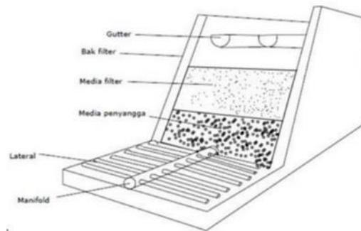
**Gambar 2. 28** Bagian-bagian filter
