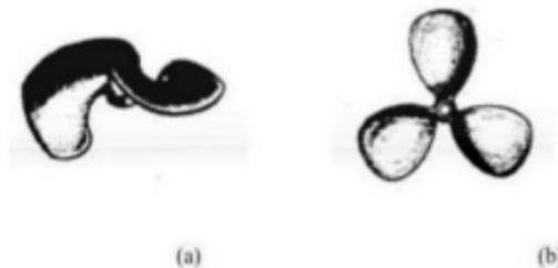
**Gambar 2. 22** Tipe Propeller: (a) 2 blade; (b) 3 blade
