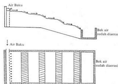
**Gambar 2. 15** *Submerged Cascade Aerator*
