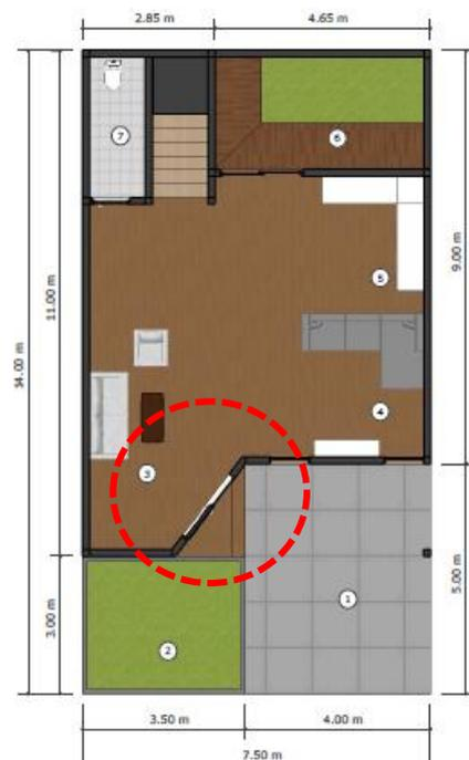
Gambar 3. 4 Final Desain denah type 100 Lt.1
