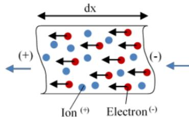
Figure 5. Movement of electrons when a potential occurs
