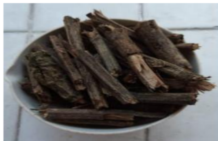
Fig. 1. Teak branches before the carbonization process
