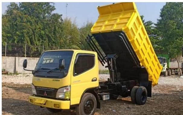
Gambar 2.8 *Dump Truck (Tipper Truck)* ukuran 6 m<sup>3</sup>
