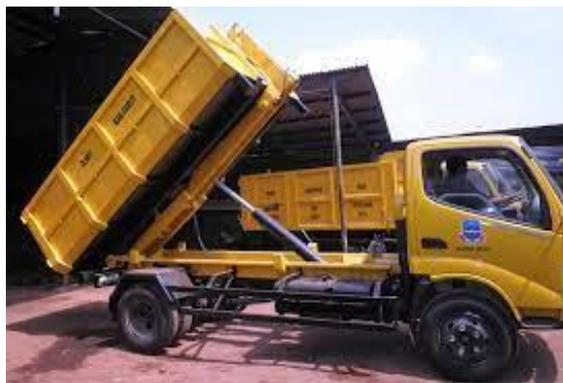
Gambar 2.9 *Arm Roll Truck* Kapasitas 10 m<sup>3</sup>
