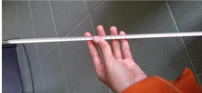
Gambar II.12 Termometer Armored Case
