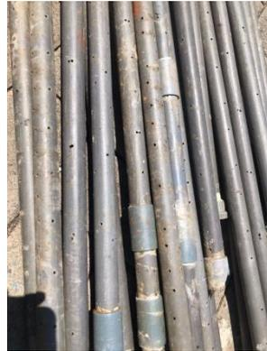
Gambar 5. 10 Perforated Tubing
