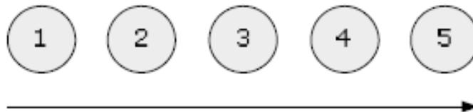
Gambar 2.2 Pola Aliran Bahan *Straight Line*
