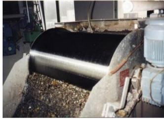
**Gambar 2.4. Rotary Drum Screen**
