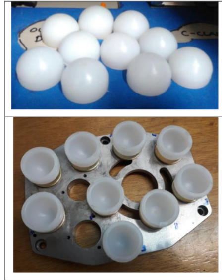
Figure 2. Acetabular Liner UHMWPE result from CNC milling
