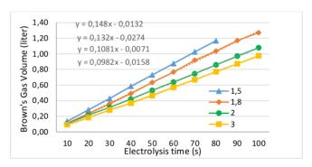
Figure 4. The comparison between the volume of Brown's gas and electrolysis time
