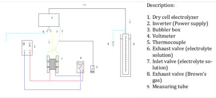
Figure 3. The installation of the experiment
