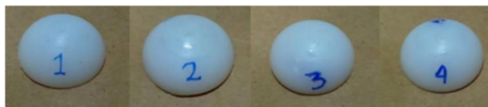
Figure 1. Acetabular liner specimen with crosslink 50 kGy (1 and 3), 100 kGy (2 and 4).
