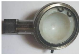
Figure 3. Setting acetabular liner on the tribometer machine chamber element.
