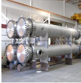
Gambar 35. Mesin Shell and Tube Heat Exchanger Sumber: (PT. Ajinomoto Indonesia, 2020)
