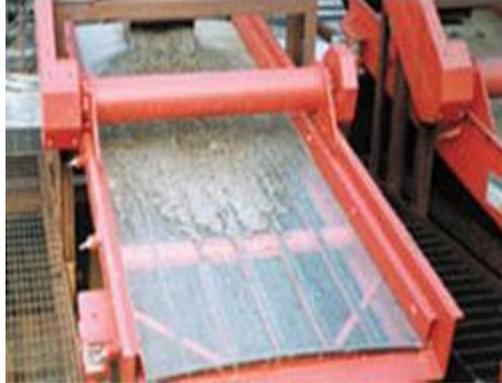
**Gambar 2.4** *Inclined screen*
