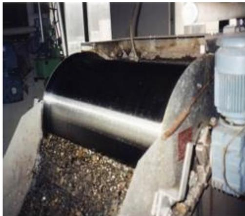
**Gambar 2.5** *Rotary drum screen*
