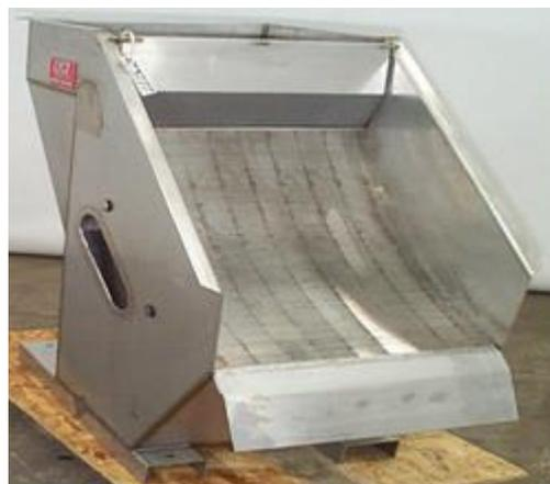
**Gambar 2.6** *Fixed Parabolic screen*
