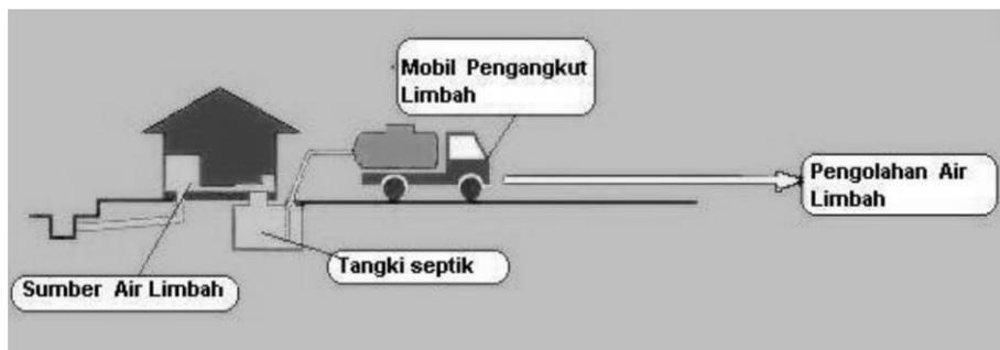
**Gambar 2.8** Diagram Sistem Pengolahan Limbah Tinja Setempat (on site)
