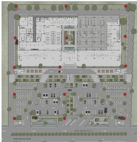
Gambar 6.13 Denah Hydrant Pillar
