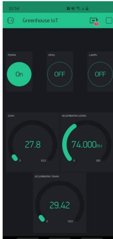
**Gambar 4. 23** Tombol Pada Output Pompa Air
