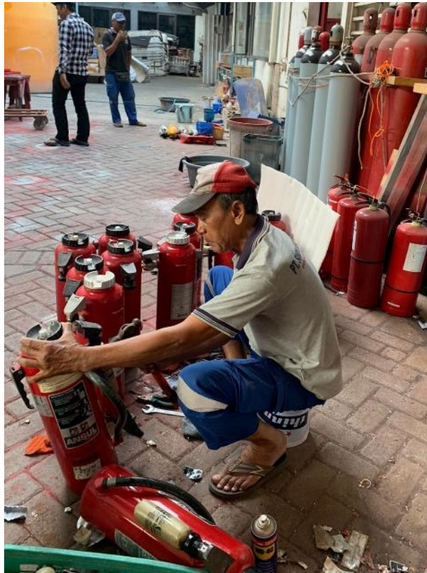
Gambar 1.2 Proses Servis APAR
