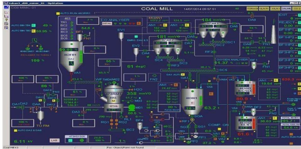
Gambar 3.15 Flowsheet Coal Mill CCR Tuban 1
