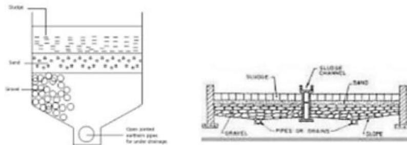
**Gambar 2.27** *Sludge Drying Bed*
