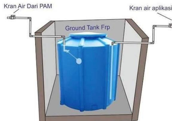
Gambar 2.18 Reservoir *Fiberglass*
