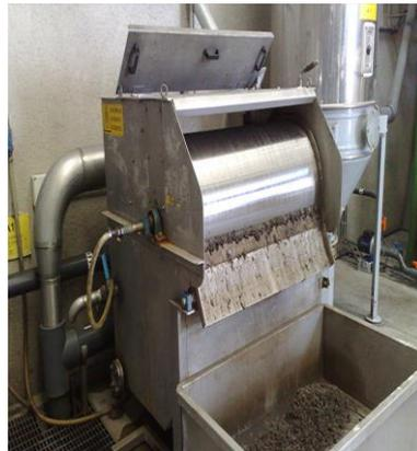
**Gambar 2.3** Drum Putar (*Rotary Drum*)
